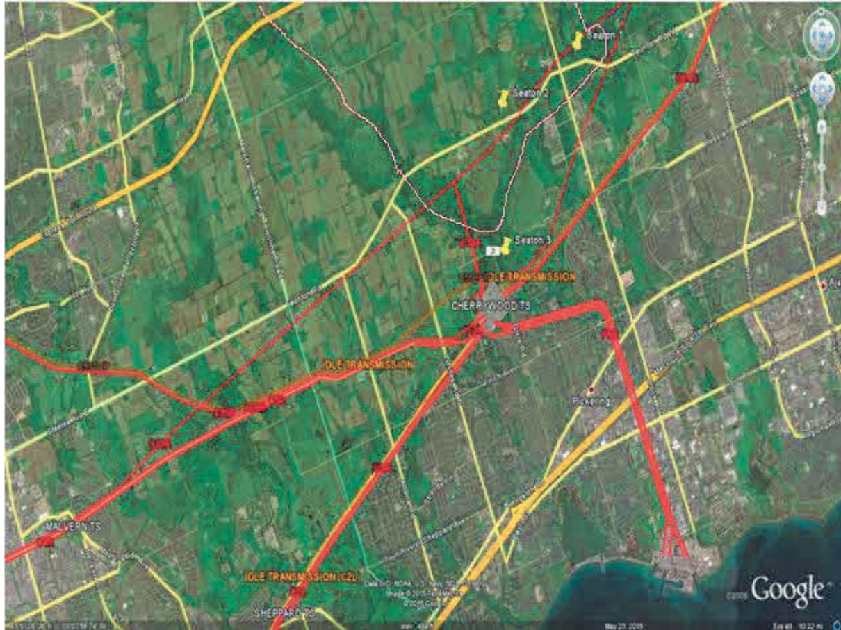
Figure 5 Locations of Alternative Sources of 27.6 kV Supply
