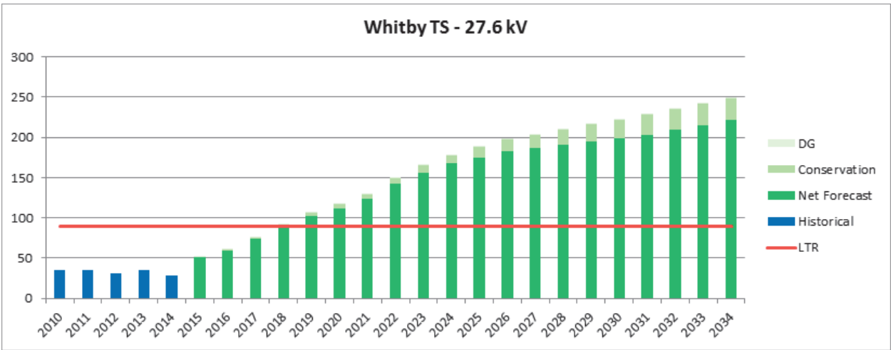
Figure 6-3: Planning Forecast for Whitby TS 27.6 kV
